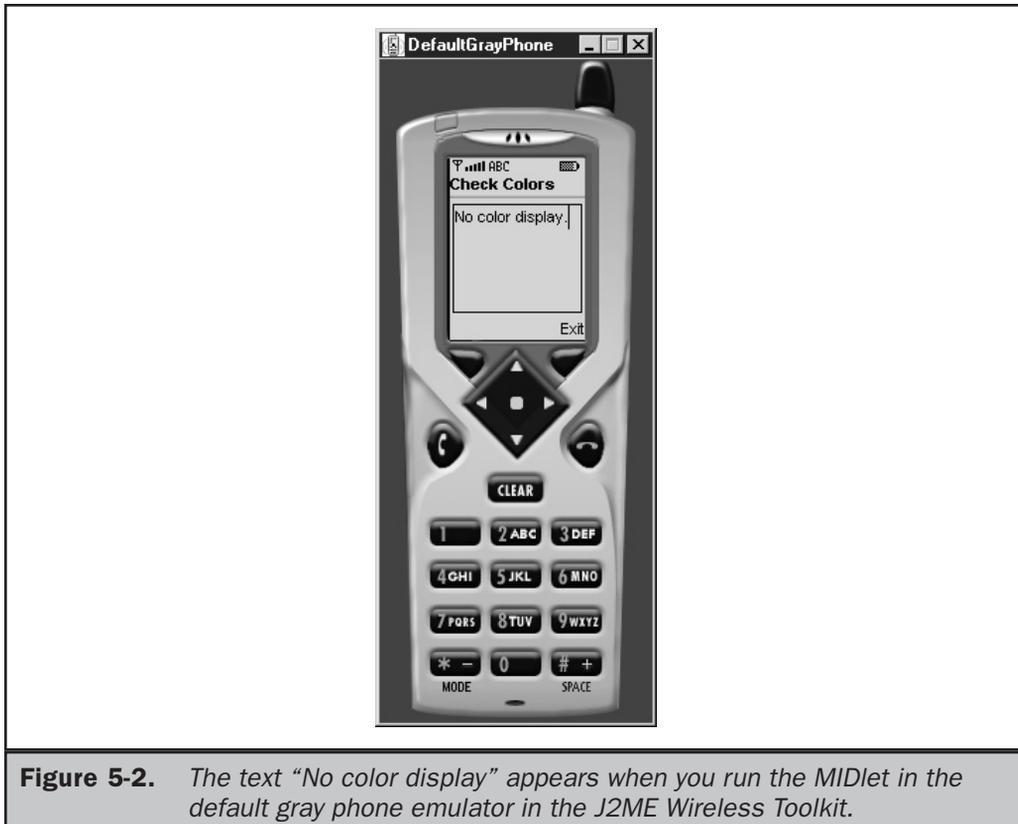
**Figure 5-2.** The text “No color display” appears when you run the MIDlet in the default gray phone emulator in the J2ME Wireless Toolkit.
