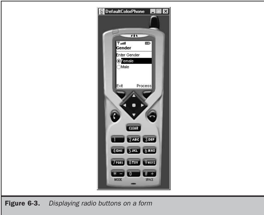
**Figure 6-3.** *Displaying radio buttons on a form*
