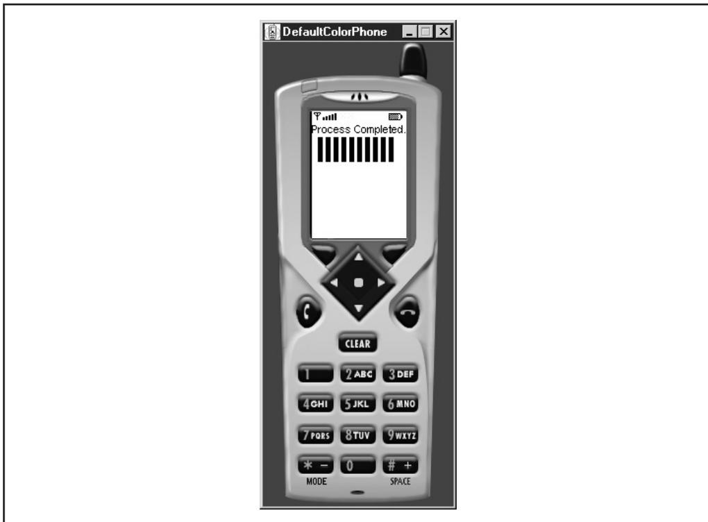
**Figure 6-5.** *Displaying a noninteractive gauge on a form*
