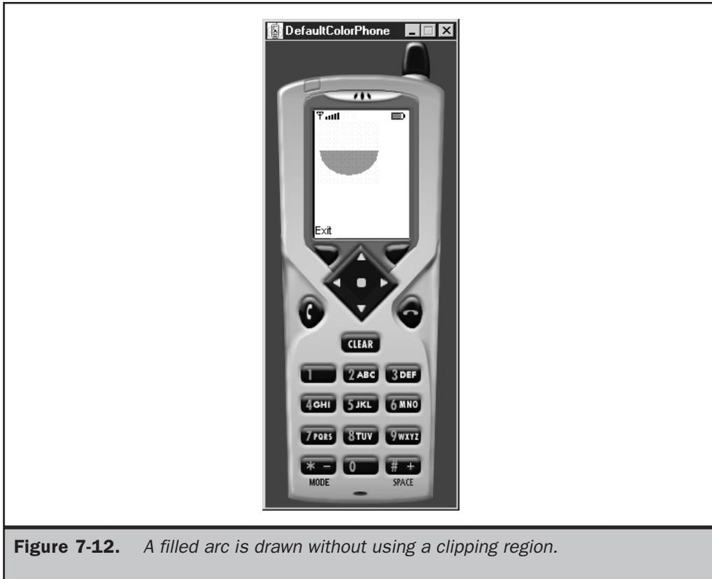
**Figure 7-12.** *A filled arc is drawn without using a clipping region.*
